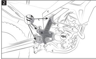
Mount the Acerbis X-Grip (A) using the original screw (E) and tighten it using the O-Rings (C) and (D). Montare l'X-Grip Acerbis (A) riutilizzando la vite originale (E) e
