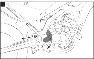
Remove the original cover by loosening the screw (E). Rimuovere la cover originale svitando la vite (E).
